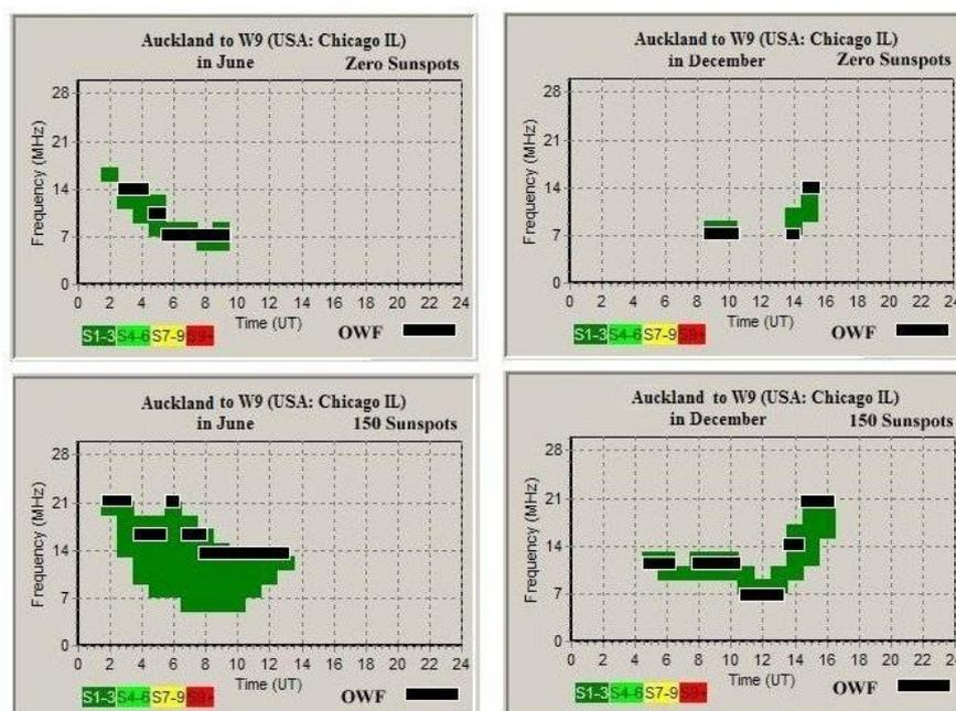
The colour bands on these graphs represent received signal strength. Dark green is a strength of 1 – 3 (very weak signals), Light Green is Strengths 4 – 7 (good signal levels) and Yellow represents strengths 7 – 9 (strong signals)
