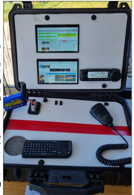
The working 100W deployable HF digi-box.
