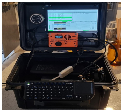
(tr)uSDX with audio to the PC through a USB soundcard. Keyboard and screen fitted to protective box, running WSJT-X on FT8. Fully self contained and powered by USB powerbank
