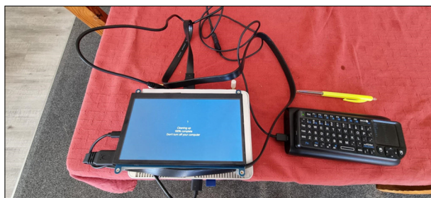
The mini-PC and 7" USB powered screen with Bluetooth keyboard & mouse. Running off a 12v USB powerbank.
