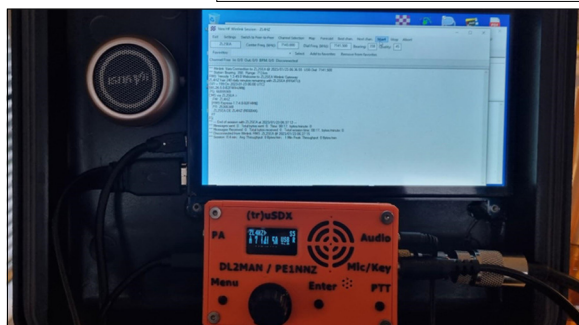
Running winlink to check email and pull down weather updates from remote locations
