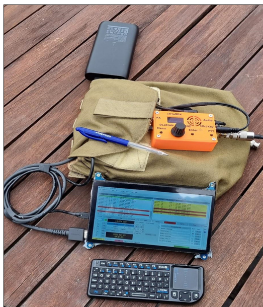
Current preferred configuration. Mini PC remains in the bag, power supply, screen and keyboard visible, FT8 QSOs to USA on 5w. Ballpoint pen for scale.
