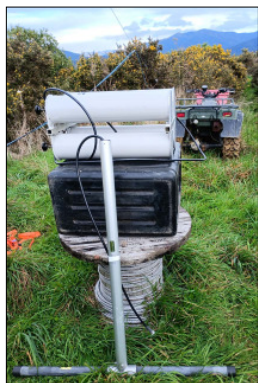
Kaikoura 690 repeater in "rack pod" transport case
