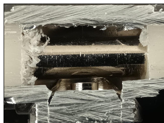
Inside open circuit tee
