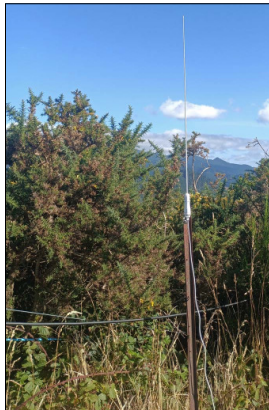
690 separate receive antenna because no duplexer
