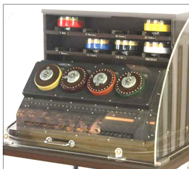
TypeX was a British coding machine modified to work like Enigmas. Unlike Enigma, the TypeX was never 'broken'.
