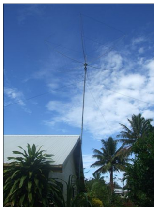
The K4KIO Hex Beam is rotated with a Yaesu G450A is mounted on a 38 foot steel mast tied.
