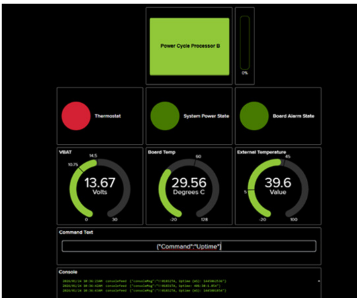
Figure 3, Remote Control of Processor B. The external temperature is the transceiver heatsink temperature
